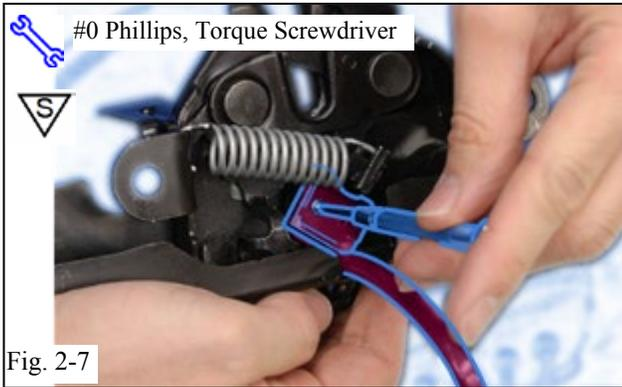
(i) Install the Hood Switch with the Switch Lever underneath the Hood Lock Trigger Lever. (Fig. 2-7)
