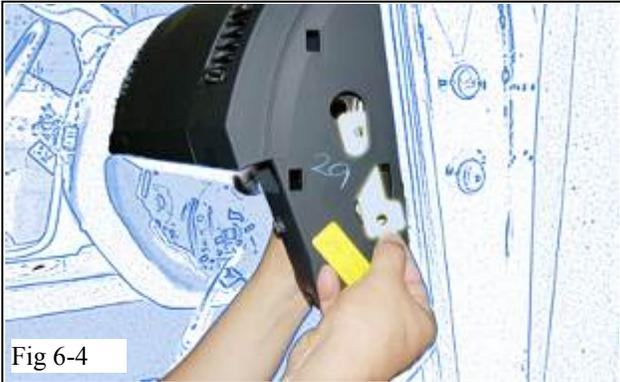
(e) Insert the RES ECU Mounting Plate through the Hole on the side of the Dash. (Fig. 6-4)
