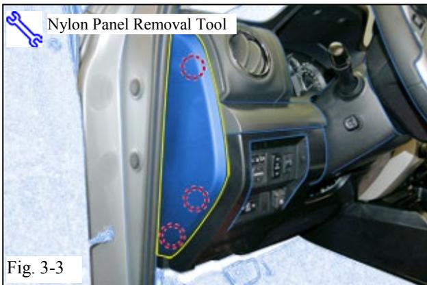
(c) Remove the Driver's Dash Side Cover. (Fig. 3-3)
