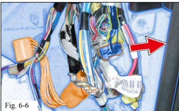
(h) Disconnect the Vehicle 22P Gray Connector from the connector block in the Passenger Cowl Area (Fig. 6-6)
