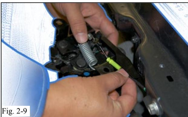
(k) Reinstall the Hood Latch Cable to the Hood Latch Assembly. (Fig. 2-9)
